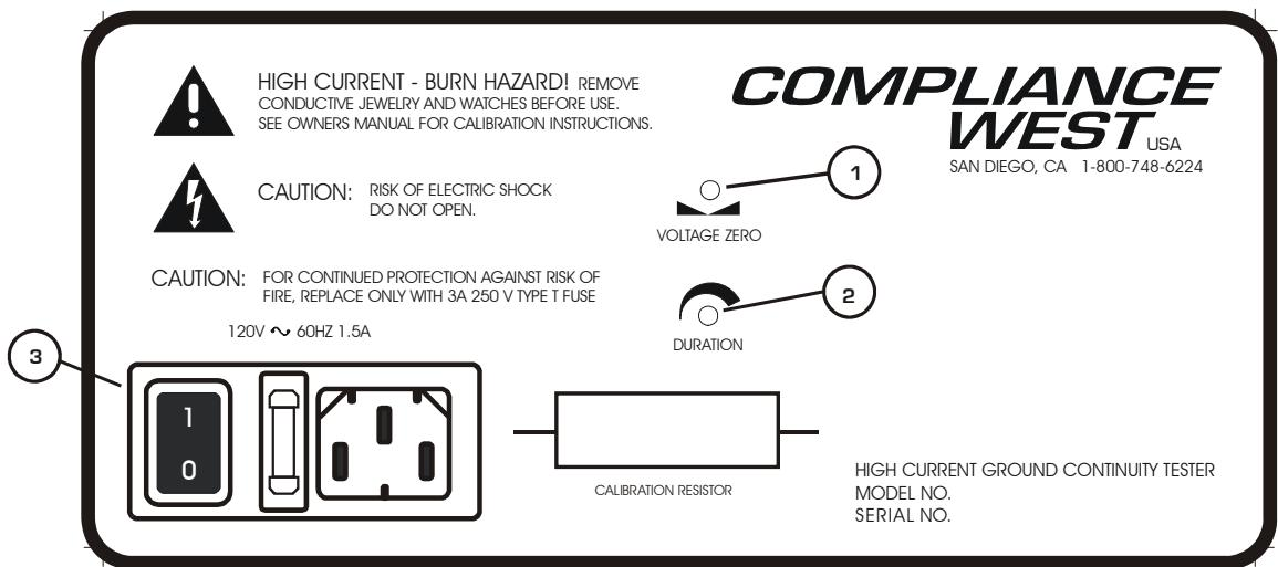
**Figure 2-2. Controls, Indicators, Connectors - Model GFM-40ac Rear Panel**
